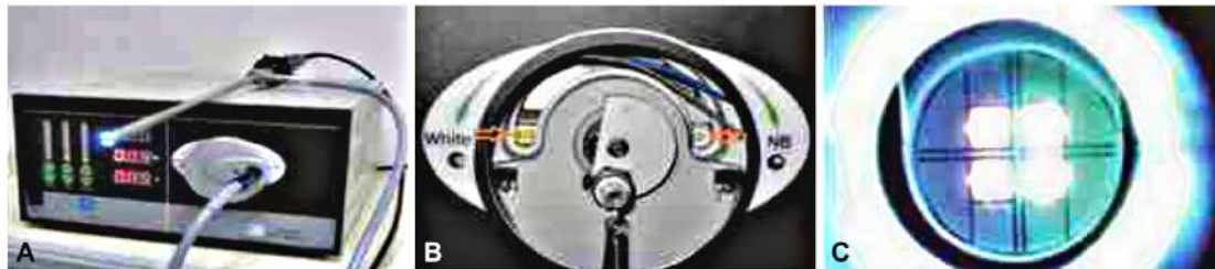
Fig. 2. (A) Light-emitting diode (LED)-narrow band imaging light source PR650, cursors for 0% to 100% white, green/blue light mix. (B) Left ⇨: white LED chip; right ⇨: green/blue LED chips. (C) Close-up view: green/blue LED chips.
